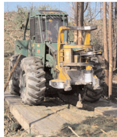
Portable bridge used to protect water quality.
